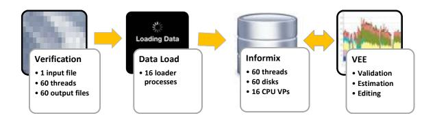
Figure 2 - Software architecture and flow for processing meter data
