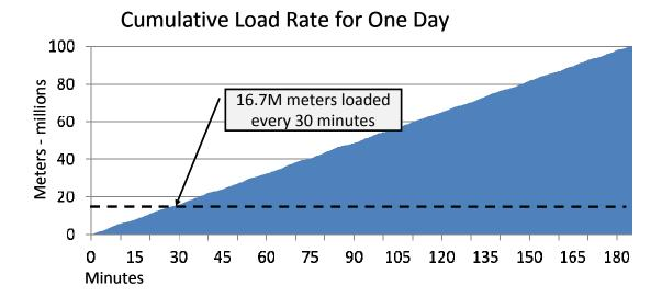
Figure 3 -Data load results for 100 million meters for one day
