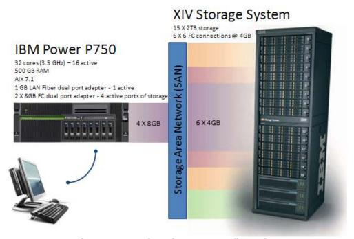
Figure 1 - Benchmark system configuration
